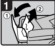
1. Open the cover of the auto document feeder (ADF) and remove the misfed original.
